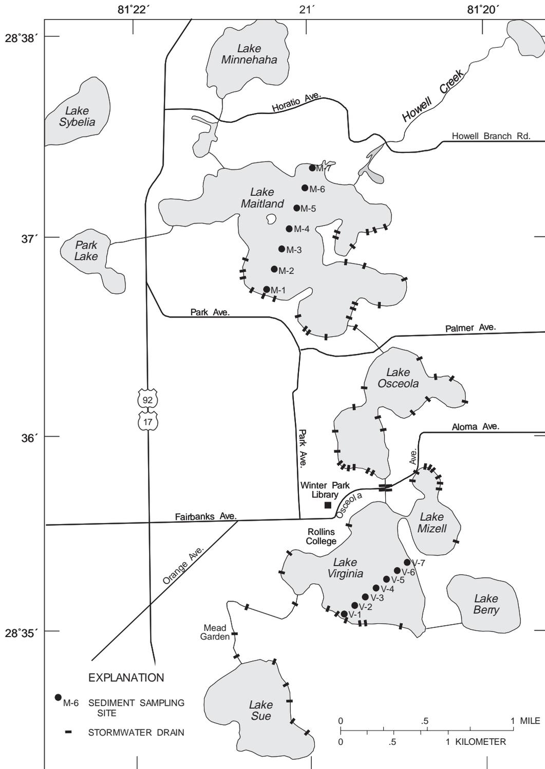
**Figure 3.** Bottom-sediment sampling sites and location of stormwater drains.
