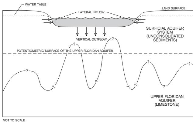
**Figure 10.** Relation of water table to potentiometric surface of the Upper Floridan aquifer and components of ground-water flow.
