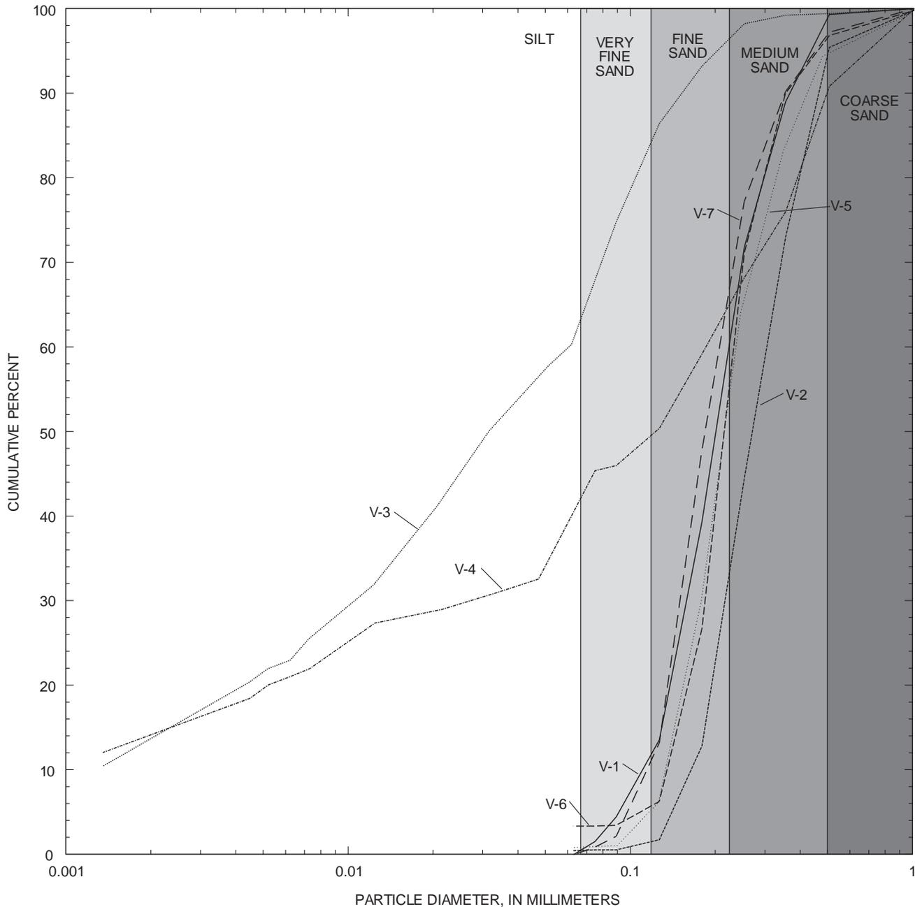
**Figure 5.** Lake Virginia bottom-sediment size distribution based on sieve and hydrometer analysis, October 1991 (site numbers are from fig. 3).
