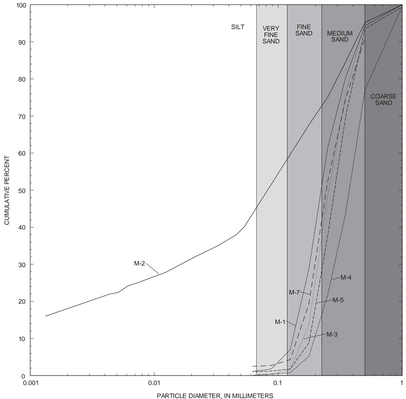
**Figure 4.** Lake Maitland bottom-sediment size distribution based on sieve and hydrometer analysis, October 1991 (site numbers are from fig. 3).
